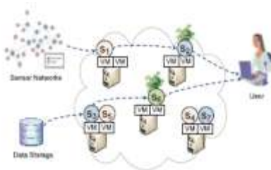
Fig. 1. Service integrity attack in cloud-based data processing. S_i denotes different service component and VM denotes virtual machines.
